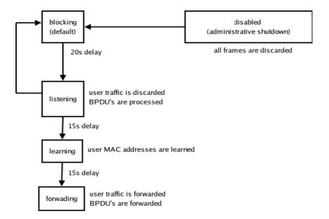
After about 50s every port on a switch is placed either in forwarding or blocking state, thus creating a logical, loop-free topology. During the election process each switch sends and receives BPDUs and processes received BPDUs to determine the root bridge. A BPDU looks like this (in C language):
