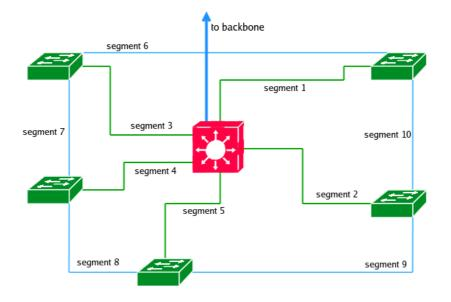
If a physical link between the Layer 3 Switch (red) and a Layer 2 Switch (green) fails, this redundant network topology will remain operational
