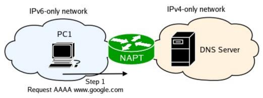
NAT-PT captures the packet and creates a new binding between the IPv6 address of PC1 and one of the IPv4 addresses it has in its pool, and translates the packet. NAT-PT sees a DNS query and translates the AAAA request to an A request. Finally it finds a route for the newly created IPv4 packet and queues it to the appropriate outbound interface.
