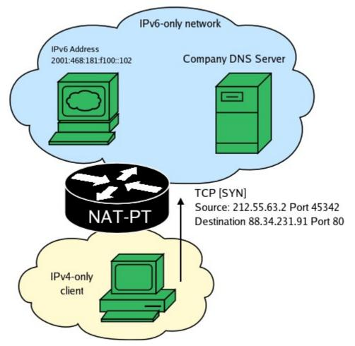
NAT-PT attempts to perform a reverse DNS resolution on the packet's destination. This is handeled by a separate thread while all other packets are being continously translated.
