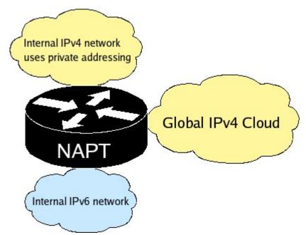
If your network topology resembles the one above, you can still use the IP address of the outside interface on the side of the global IPv4 cloud. You can do this by entering it a IP pool range containing only one IP, this is explained in more detail below.
