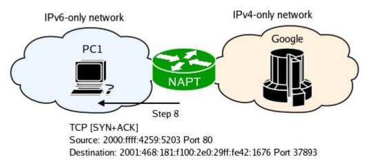
The above summarizes the basics of how IPv6-only and IPv4-only hosts communicate. The rest of the connection occurs in the same way. NAT-PT maintains three "translation" pools, one for TCP, one for UDP and one for ICMP. By default TCP translations timeout after 5 minutes from the time RST or FIN packet was captured, or after 24 hours of innactivity. UDP translations expire after 1 hour, and ICMP after 30 seconds.
