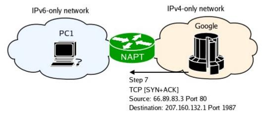
NAT-PT captures the traffic and finds a the IPv6 address for the mapping. Finally it finds a route for the newly created IPv6 packet and queues it to the appropriate outbound interface.
