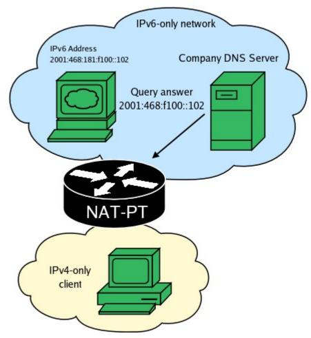
NAT-PT creates a mapping between the returned IPv6 address and the packet's original IPv4 destination, it then translates the packet and sends it to its destination.
