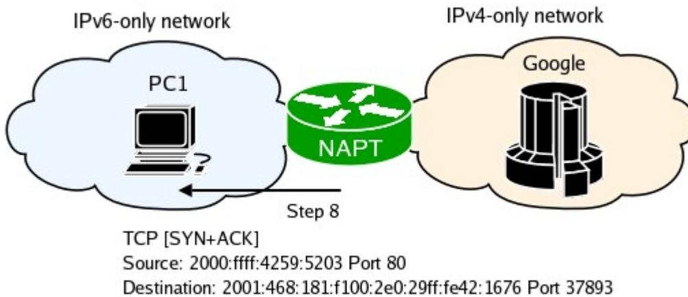
The above summarizes the basics of how IPv6-only and IPv4-only hosts communicate. The rest of the connection occurs in the same way. NAT-PT maintains three "translation" pools, one for TCP, one for UDP and one for ICMP. By default TCP translations timeout after 5 minutes from the time RST or FIN packet was captured, or after 24 hours of inactivity. UDP translations expire after 1 hour, and ICMP after 30 seconds.
