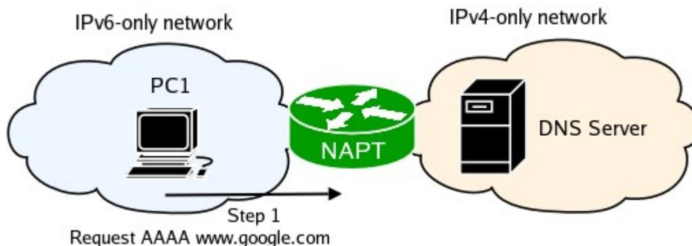
NAT-PT captures the packet and creates a new binding between the IPv6 address of PC1 and one of the IPv4 addresses it has in its pool, and translates the packet. NAT-PT sees a DNS query and translates the AAAA request to an A request. Finally it finds a route for the newly created IPv4 packet and queues it to the appropriate outbound interface.
