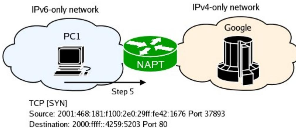
NAT-PT captures the packet and creates a new binding between the IPv6 address of PC1 and one of the IPv4 addresses it has in its pool, translates the packet, finds the route, and ...etc.
