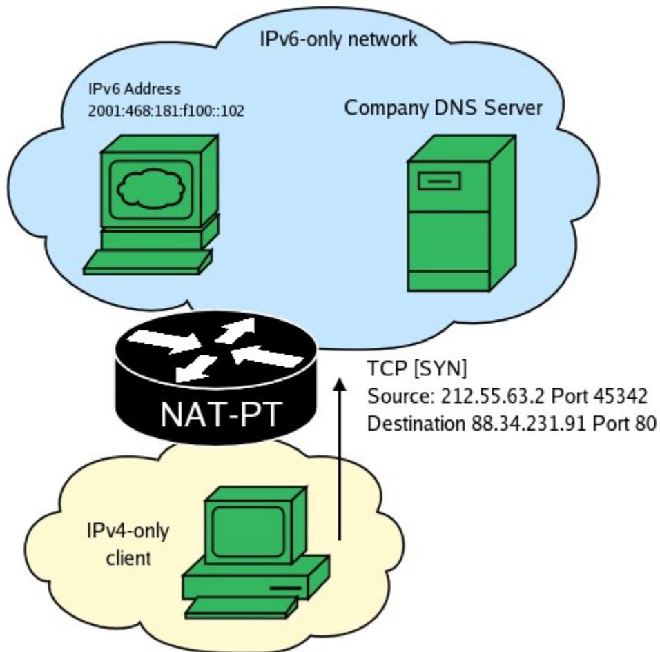
NAT-PT attempts to perform a reverse DNS resolution on the packet's destination. This is handled by a separate thread while all other packets are being continuously translated.
