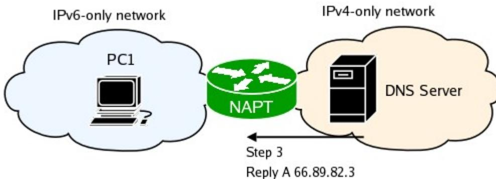
NAT-PT captures the traffic and finds a the IPv6 address for the mapping. It also sees the DNS A resource records and translates them to AAAA records. It does this by adding a special 'NAT-PT prefix' (configured through 'naptd-confmaker', default 2000:ffff:.) to the beginning of the IPv4 address. Finally it finds a route for the newly created IPv6 packet and queues it to the appropriate outbound interface.
